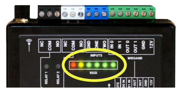
For further testing, connect a Weigand reader to the **Remote** unit, the reader should turn on during this test. Swipe a fob on the reader and look for the following:
