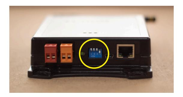
The switches allow you to configure the unit for **Central** or **Remote** operation, enable pairing mode, or set relays to be Wet or Dry. Dry relays act as simple switches that open or close a circuit without supplying power. Wet relays provide a 12VDC (1.5A Max) output to directly power devices when activated.
